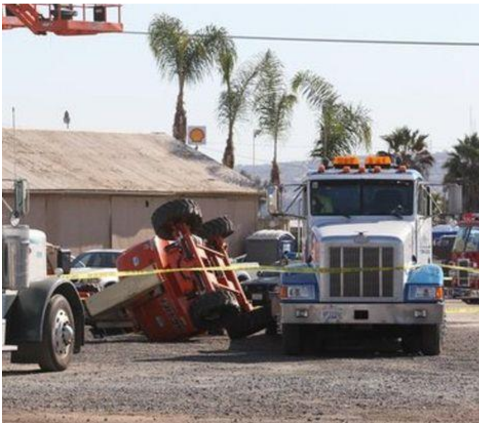
The boom slipped off the side of the low loader
